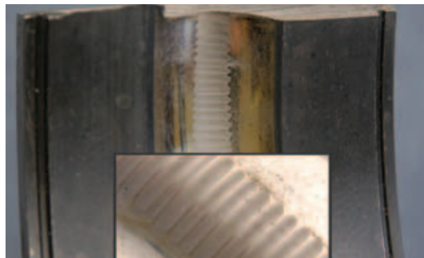
Bearing fluting, "washboard" pattern on the bearing surface
