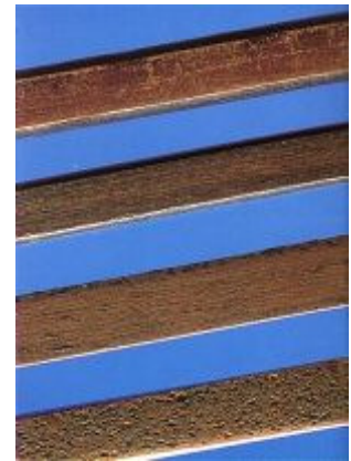
These photographs taken under a microscope show the differing wear characteristics to the overhead wire from using carbon, copper, sintered metal and aluminium as a collector material.
