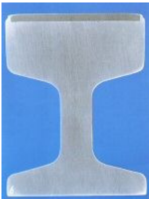
This photograph shows the potential vulnerability of modern capped third rails.
