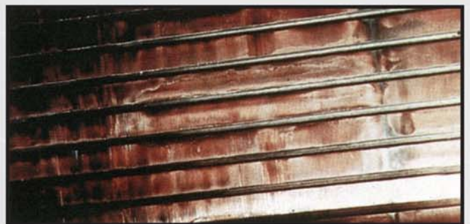
Figure 2 Mottled – Satisfactory operation can result with a film color that is not uniform.
