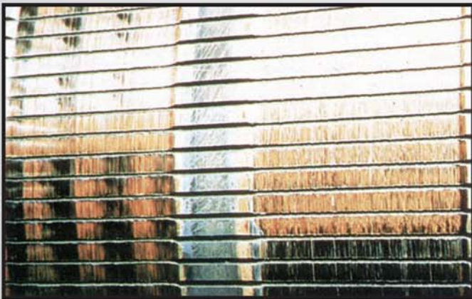
Figure 10 Grooving – Metal machined from across the brush paths.
