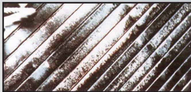
Figure 12 Nonconductive Filming – Brush sparking usually results from this condition.
